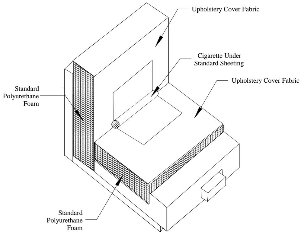
Figure C-3. Mock-up Assembly for Smoldering Ignition Resistance Test of Barrier Materials
