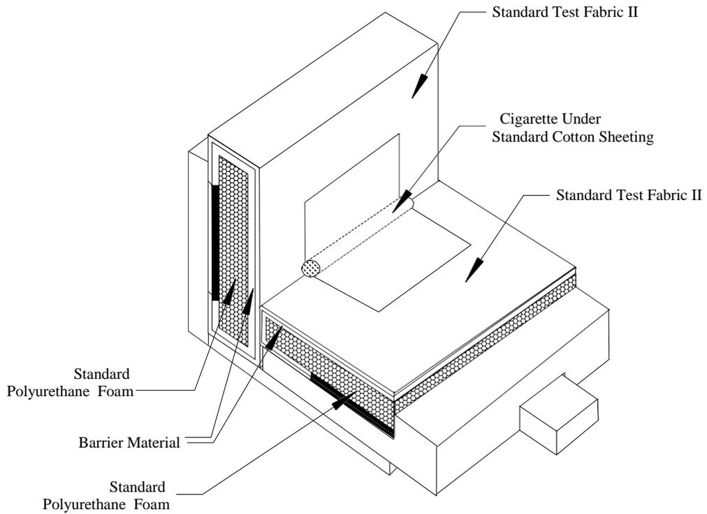
Figure C-4. Mock-up Assembly for Smoldering Ignition Resistance Test of Resilient Filling Component Materials
