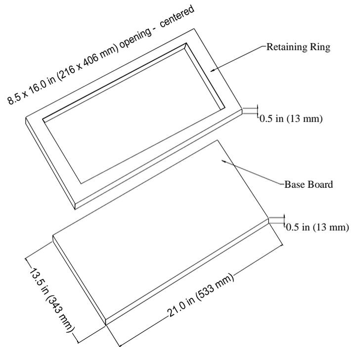
Figure C-6. Mock-up Assembly for Smoldering Ignition Resistance Test of Decking Materials.
