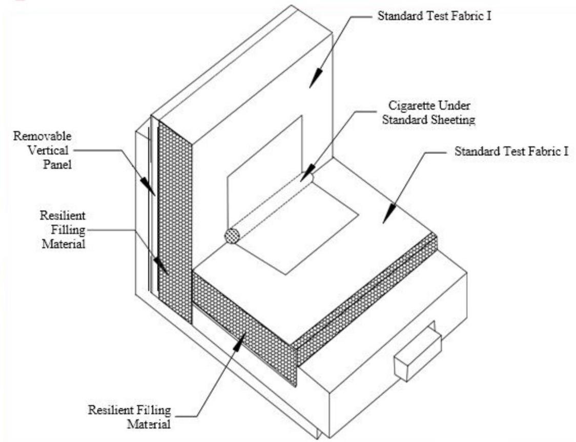
Figure C-5. Decking Materials Tester.
